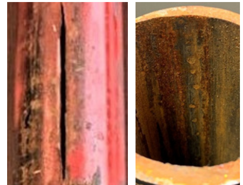
Tubing Failure and Erosion
