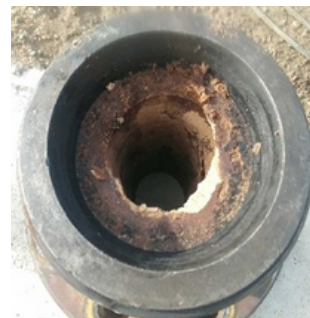
Cap Check - Regular Tubing, Wax is Hardened and Dehydrated
