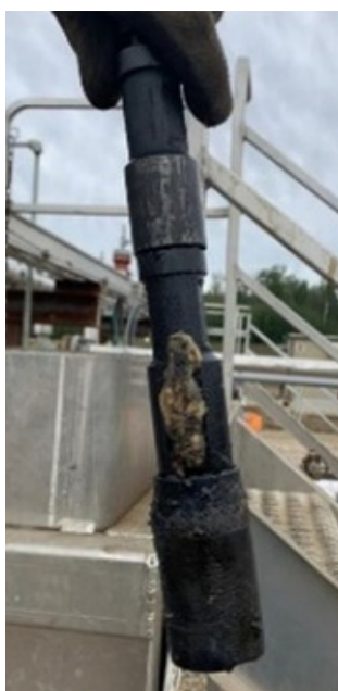
Minimal Wax on Gauge Ring, No Knives
