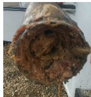
Wax Build-Up in Regular Tubing String After 10 Days
