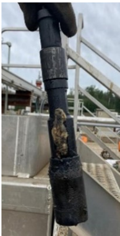
Minimal Wax on Gauge Ring, No Knives
