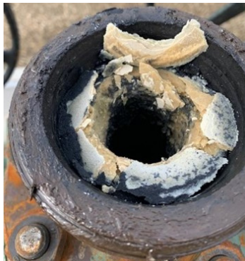
Cap Check - Coated Tubing, Wax is Soft, Not Dehydrated
